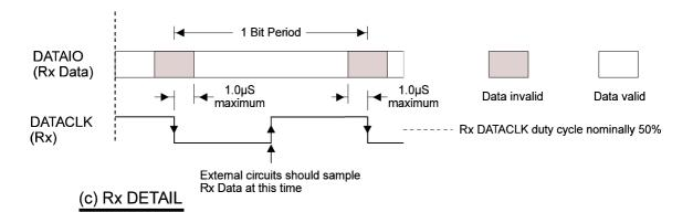
Figure 8 Tx/Rx Data and Clock Timings
