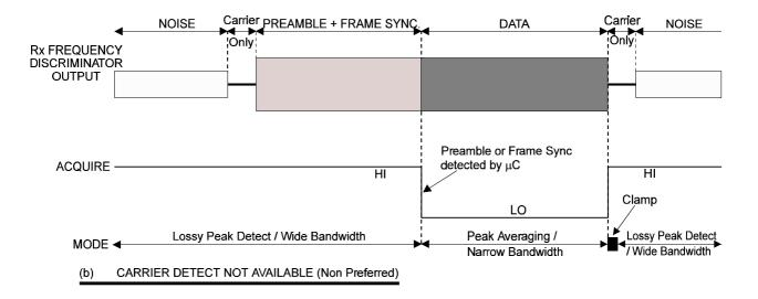
Figure 7 Receive Control Mode Diagram
