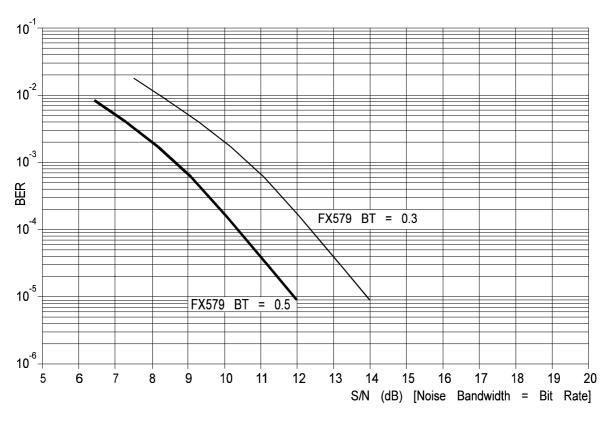
Figure 9 Typical Bit Error Rate Performance
