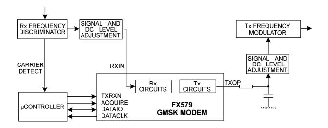
Figure 3 Typical Radio Application
