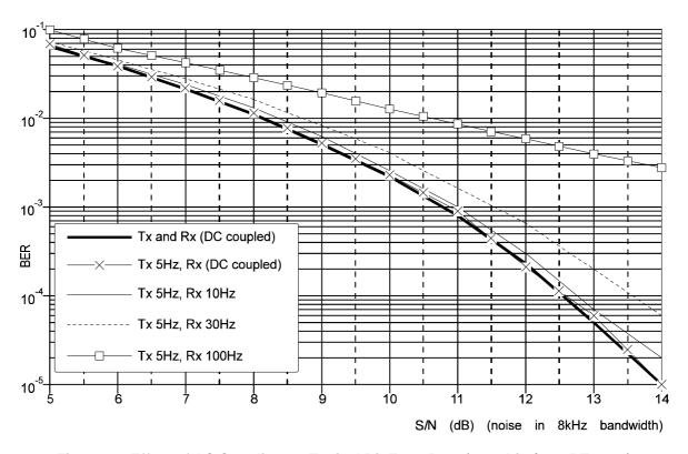
Figure 10 Effect of AC Coupling on Typical Bit Error Rate (8000 bits/sec, BT = 0.3)
